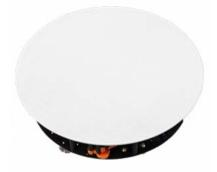
Round speaker for either in-wall or in-ceiling mount, 5,25" coaxial driver 0.75" titanium dome tweeter tiltinge and built-in 100 V transformer with 16-8-4-2 W power taps. 120° wide coverage. ABS chassis and stainless steel round protection grille painted in white or black.
