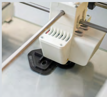
3D printed prototypes are a fast and convenient part of the design process
